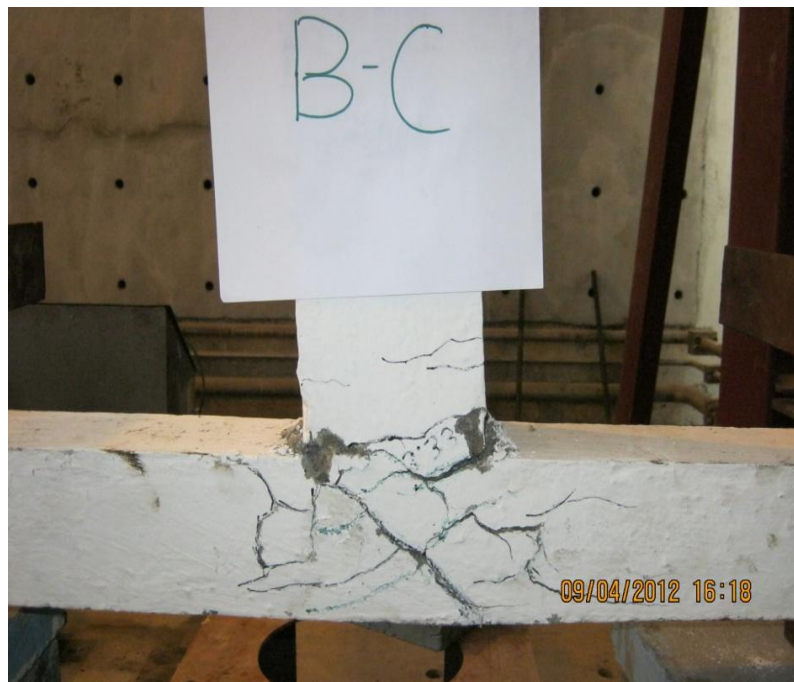
Figure 6. Cracks on RCBC joint specimen at the end of testing
